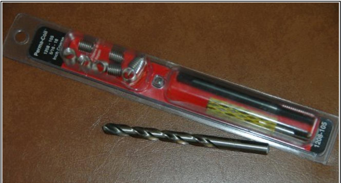
The kit consists of a dozen of the helicoil inserts, the special tap and the insertion tool. (The yellow in the picture is a plastic sleeve to protect the threads of the tap when not in use.) The kit for the 5/16-18 insert was about \$22 and the drill bit was about \$5.
