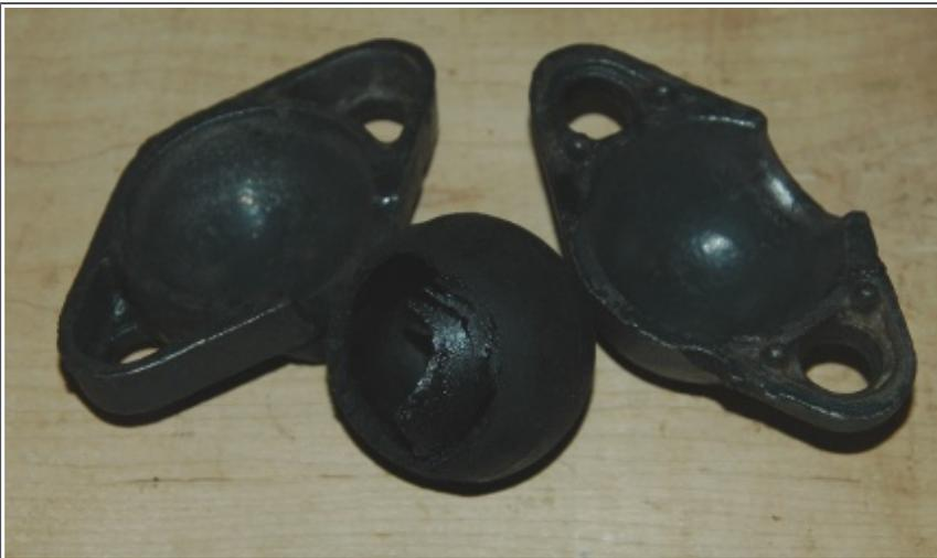
The inside diameter of the cast iron cup cavity is 1.850”. This dimension was measured at the opening of each piece as well as by measuring the depth of each piece and adding.
