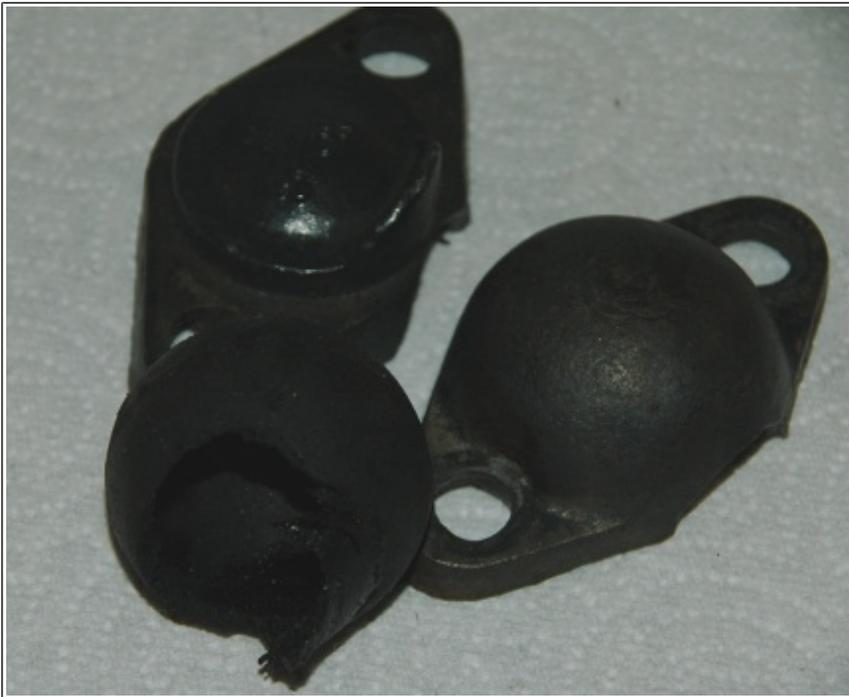
Taking off the nuts on the radius ball cap, I discovered several things. First, there were no cotter pins, no spacers, no springs, and the caps were cast iron. Inside the caps, the ball was encased in a rubber ball.
