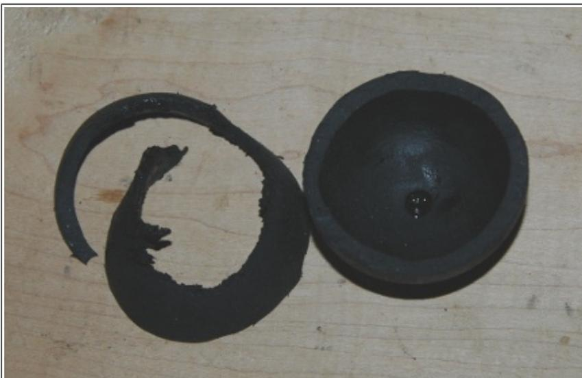
I did a bit of analysis of the rubber ball and the cast iron caps. I cut the ball around the circumference at the mold line that was still visible on the ball. Looking at the pieces, you can see that the ball is noticeably thinned on the left side in the picture, and that corresponds to the totally disintegrated area that was the front half of the ball. In the picture, the area of the rubber that was on the bottom of the radius ball is at the left of each piece.
