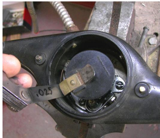
Another thing often overlooked is the gap between the rotor and the nibs inside the distributor body. The gap should be set at .025 and all four gaps should be the same. Measure each gap and file the nibs until you get .025 on all four. If you have over .025 carefully bend the metal tab on the rotor upward, then remeasure and refile if necessary. Inconsistent gaps will give you inconsistent fire at the spark plug. The gap here is as critical as the point gap.
