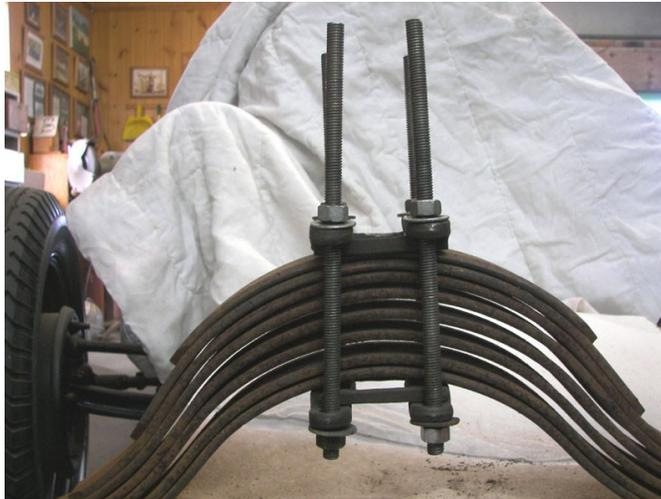
Second picture is the spring being un compressed. You slowly and carefully, a little at the time, release each of the nuts of the threaded rod one corner at the time.
