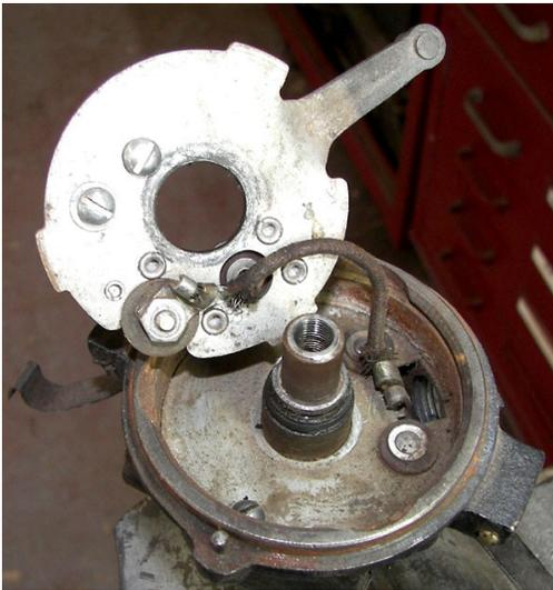
If you look carefully at the picture above you can see a broken end of the pigtail wire where it connects to the bottom of the points ---diaaster
