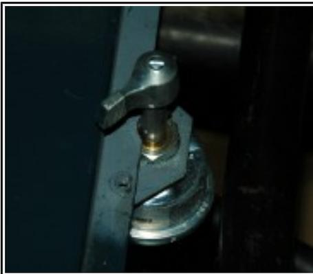
The switch was mounted so that it extended through the front edge of the center floor board on my A. That positions it at the back edge of the body cross member and just in front of the Emergency Brake Cross Shaft. Note that I had to make a small notch on the body cross member to give me clearance.
