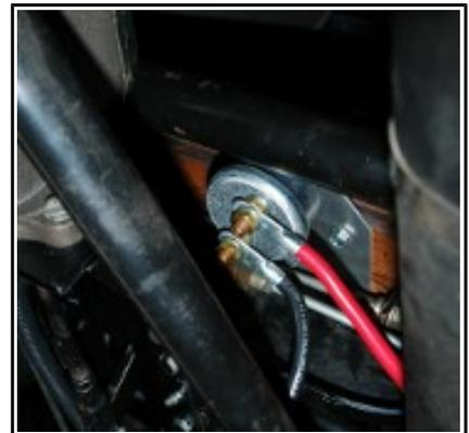
The switch was mounted to a piece of 3/32” aluminum sheet that I shaped to fit. It is attached to the bottom of the wooden cross member under the body cross member.
