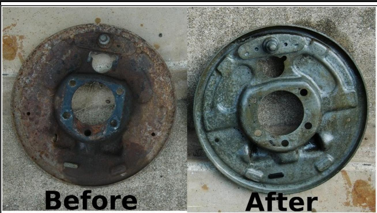
The backing plates were NOT cleaned thoroughly before I dumped them in. And anyplace there was a lot of grease or remnants of paint, the mixture didn't clean. But after a month or so (I forgot them!), they really cleaned up nicely. I used a high pressure sprayer to wash them off after their long soak, and the remnant paint just blew off the steel.
