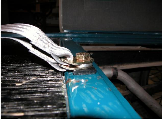
Between the two belts I used three of the flat washers to space the two belts apart just a bit so that the fabric of the belts would not interfere with tightening the belts down.
