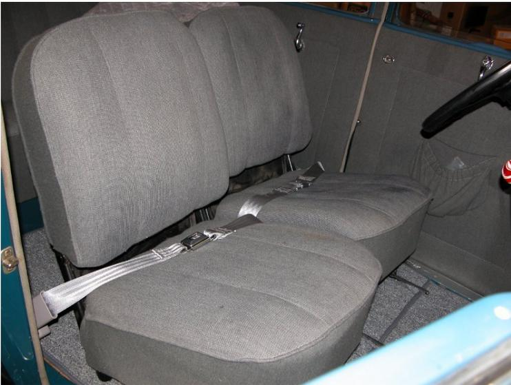
Once you have the seats back in, have someone sit in each seat and adjust the angle of the retractors so that the belt pulls straight out of the unit, then tighten their attachment bolts.
